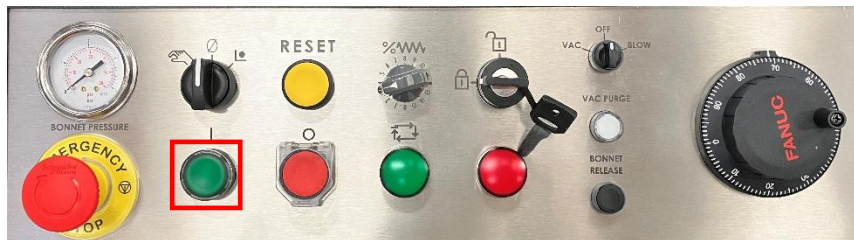
Figure 12 - CNC Drives ON switch
